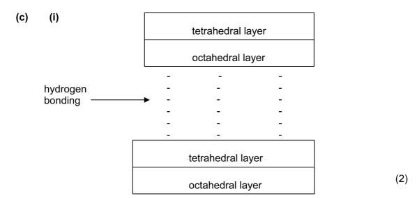
(ii) Water cannot enter the gap between the layers due to hydrogen bonding between them (1)
