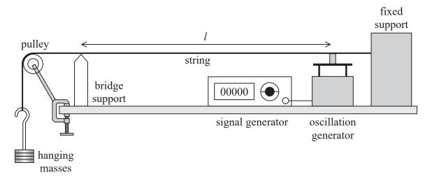
When the signal generator is switched on the string oscillates. The signal generator can be adjusted so that the string resonates.
