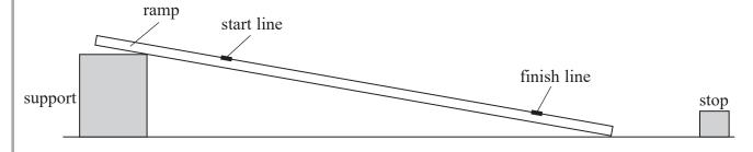
(a) (i) By placing the cylinder at the start line, take an accurate measurement of the time taken *t* for the cylinder to roll to the finish line.
